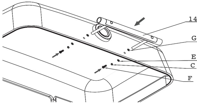
Angle the assembly slightly to the back and remove both M6x20mm screws, then do the same at the front, supporting the parts so they don't drop. Keep all of the fasteners for later use. Removable stickers at the front and rear will mark the positions of these screws. Remove the hood and barbecue chassis assembly from the stand top and place on the ground.
